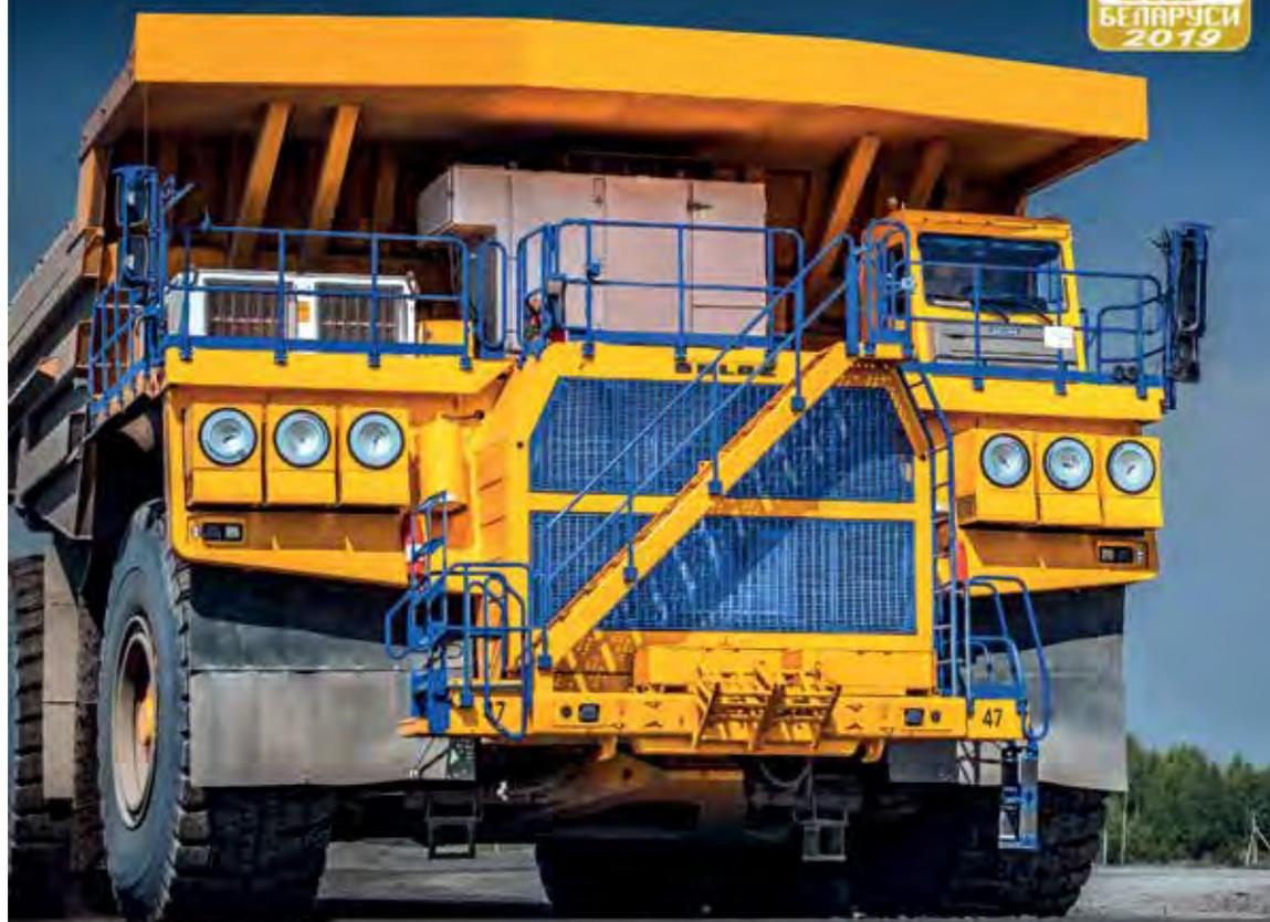
Mining dump truck **BELAZ-75605** with payload capacity of 360 metric tons
